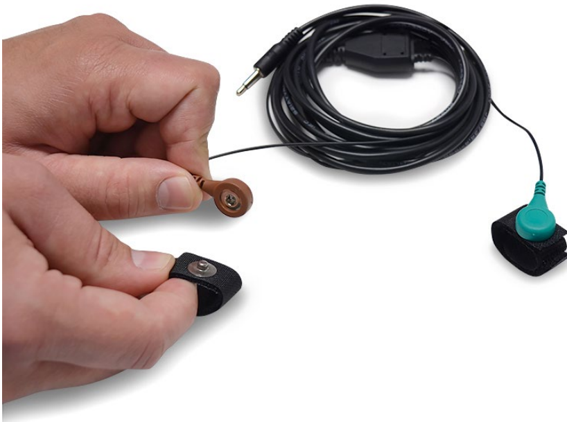
Figure: GSR connecting GSR electrodes
